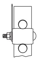
CAUTION If pipe sealant is used on threads, the degree of resistance between mating parts is less, and there is an increased chance for cracking the heat exchanger fittings. Do not overtighten.
