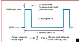
PWM levels = zero volt and 5V ( $\pm$ 3%) for 9-30V supply = zero volt and V<sub>s</sub> ( $\pm$ 1%) for 5V supply
