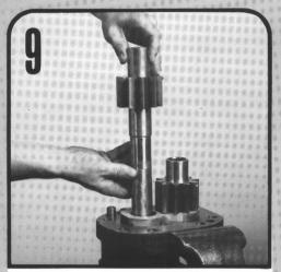
Insert the integral shaft and gear. Push down until the gear is tight against the thrust plate. Insert the matched driven gear.
