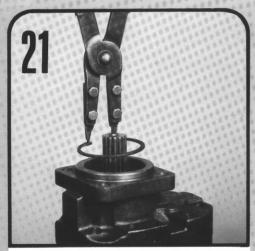
Install the snap ring in the groove.
