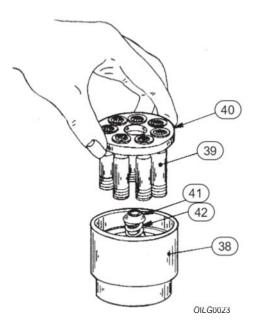
Figure 9. Rotating Group Disassembly
