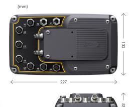
**CCpilot XA** is an ARM-based touch screen display and controller for creating a premium user experience in cost sensitive industrial vehicle applications.
