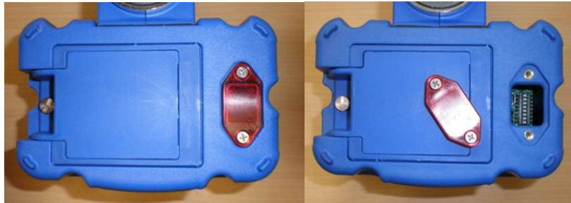
Figure 7: USB/IR Cover Location and Cover Removal
