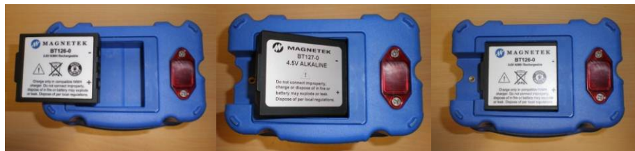
Figure 4: Installation of Battery Pack into PGT transmitter
