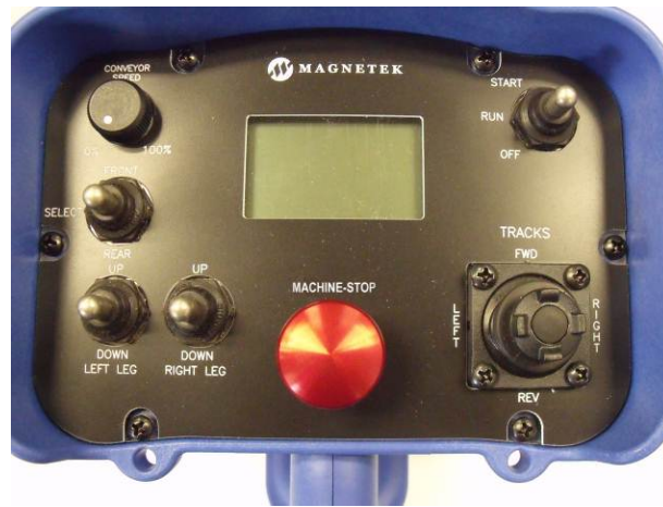
Figure 9: Machine Stop Switch and OFF-ON-START toggle
