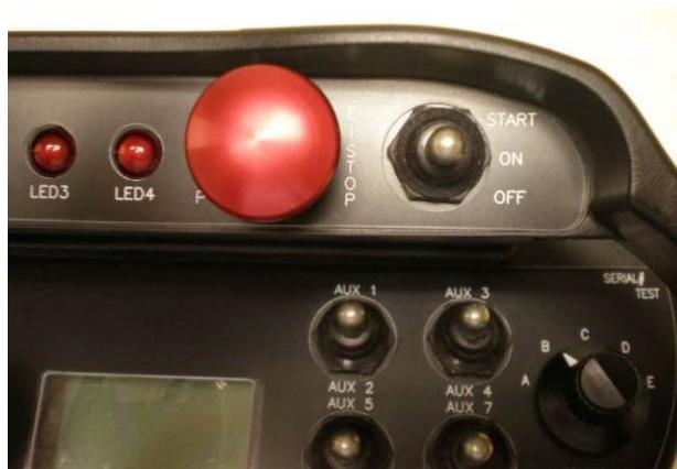
Figure 9: Machine Stop Switch and OFF-ON-START toggle
