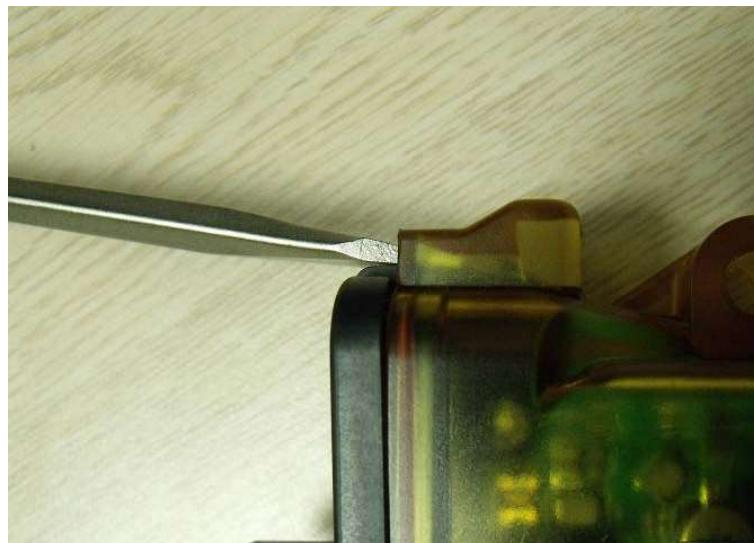
**Figure 06: CAN-2 housing removal procedure**
