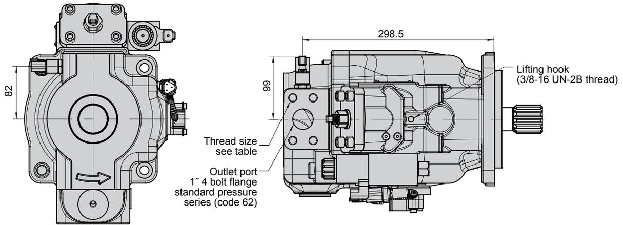
**Port option D** (pump with metric threads)
