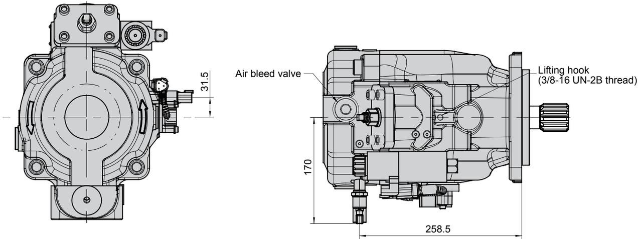
**Port option D** (pump with metric threads)
