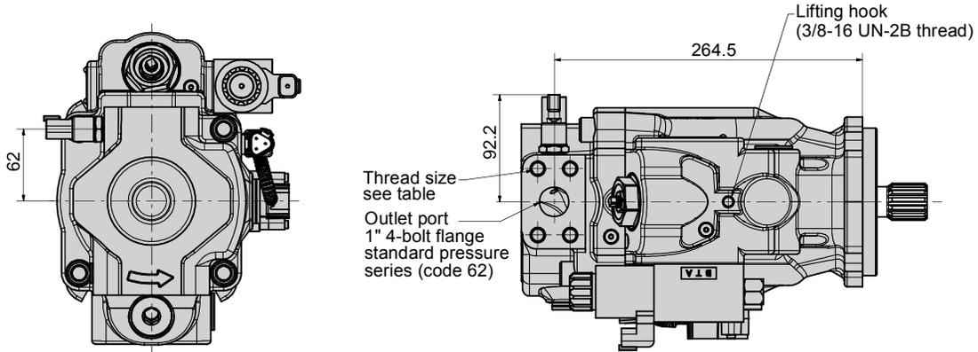
**Port option D (pump with metric threads)**
