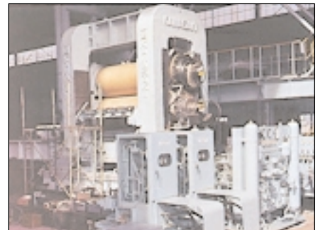
Skin Pass Mill Pump Used: K3VG112
