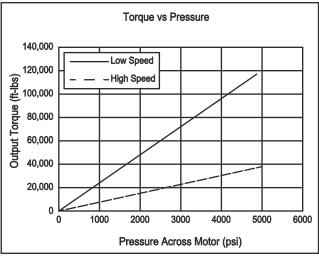
TORQUE AND SPEED CHARTS ARE BASED ON ANALYTICAL CALCULATIONS USING GEARBOX AND MOTOR EFFICIENCIES. SPEED VS. FLOW CHART SPECIFIES MAX-IMUM FLOW AND SPEED VALUES FOR THE DRIVE. STARTING TORQUES ARE APPROXIMATELY 25% LESS THAN RUNNING TORQUE. SYSTEM BACK PRESSURE WILL REDUCE THE RUNNING TORQUES PROPORTIONALLY.
