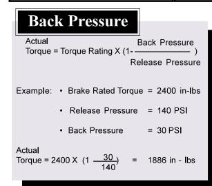
**B**ack Pressure refers to pressure existing in the discharge side of a load and is a result of fluid flow restrictions.
