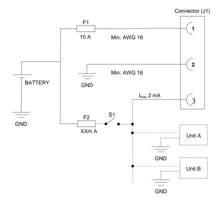
By connecting the power supply according to the illustration above, the device will automatically start when the main switch or turnkey is turned on, and shut down when the switch or turnkey is turned off.
